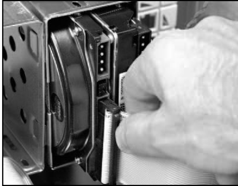
Ribbon uses parallel transmission to connect a disk drive to the motherboard
